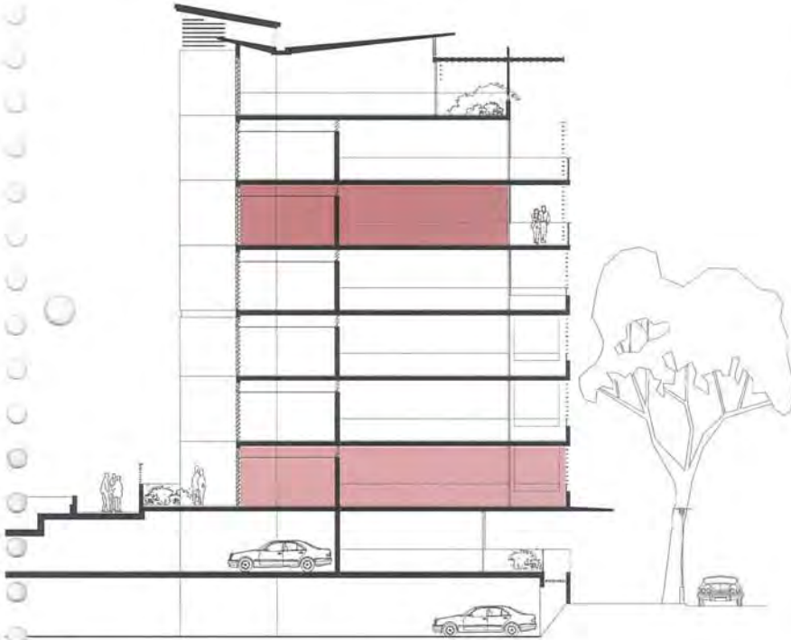
SECTION TYPICAL HIGH RISE APARTMENTS 1:250
